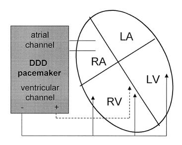
AV resynchronization 13/20(1°AVB10, CAB3) atrial synchronous univent pacing 10 atriouniventricular sequential pacing 3 AV delay – optimized to achieve highest increase in syst and mean pressure
